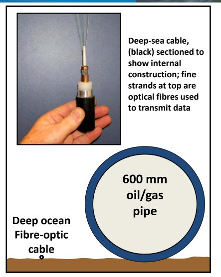
Modern fibre-optic cable in hand (for scale) and relative to 600 mm diameter subsea pipe
