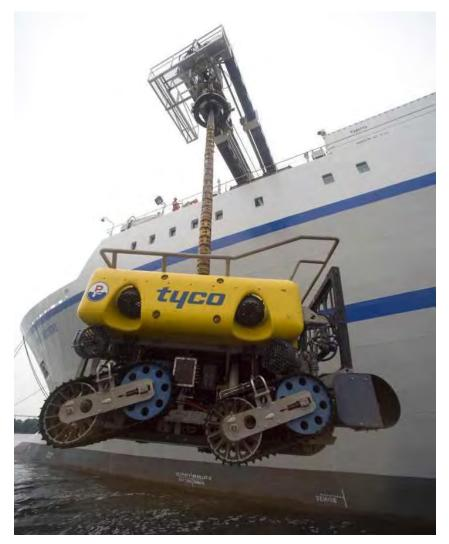
ROV used for cable inspection, recovery and burial Source: TE SubCom www.iscpc.org
