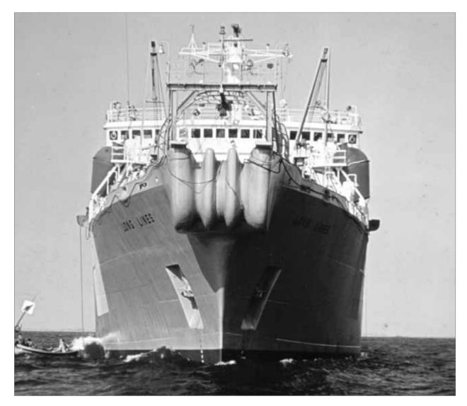
cable laying and improved methods of strengthening cables, especially in deep water where as much as 6 km of cable could be suspended through the water as it was laid on the ocean floor from a cable ship.
