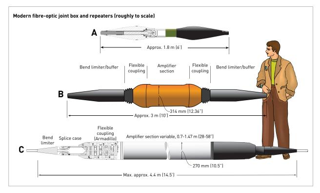
Figure 2.5: Representative repeaters from different manufacturers. The housings can accommodate as many as eight individual regenerators, or more recently, optical amplifiers. *Source: Lonnie Hagadorn.*
