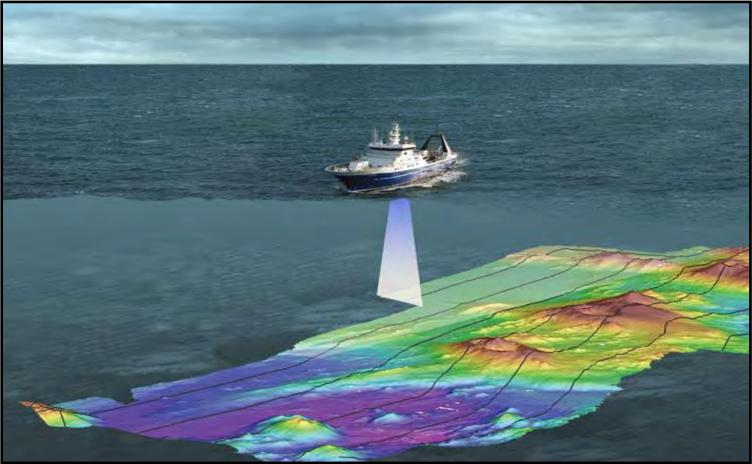
Seabed mapping systems accurately chart depth, topography, slope angles and seabed type Source: NIWA
