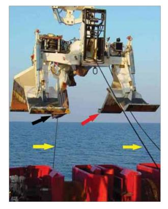
Figure 3.4: A sea plough about to be deployed from a cable ship. The fibre-optic cable (yellow arrows) is fed into a furrow cut by the plough-share (black arrow), which is towed across the seabed on skids (red arrow). Source: Alcatel Submarine Network (ASN) now Alcatel-Lucent.
