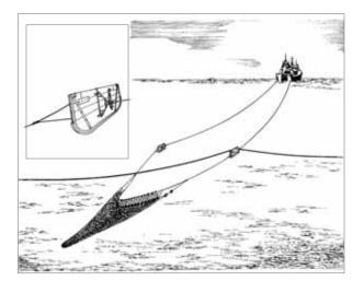
anchor on a cable (Figure 7.1), vessel stability and crew safety can be affected. In spite of extensive warnings from cable companies, there are still occasional cases of fishermen hauling cables to the deck and cutting them, risking damage and injury not only from the weight and tension on the cable, but also from the electricity used to power the repeaters (Chapter 2).
